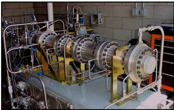
Fig. 4: The 20 MW i CES Gas Generator (GG). Combustor section is at far end followed by 4 sequential water-cooldown sections. Closest to observer is the downstream endplate that provided back-pressure during testing 'in lieu' of HP turbine.
