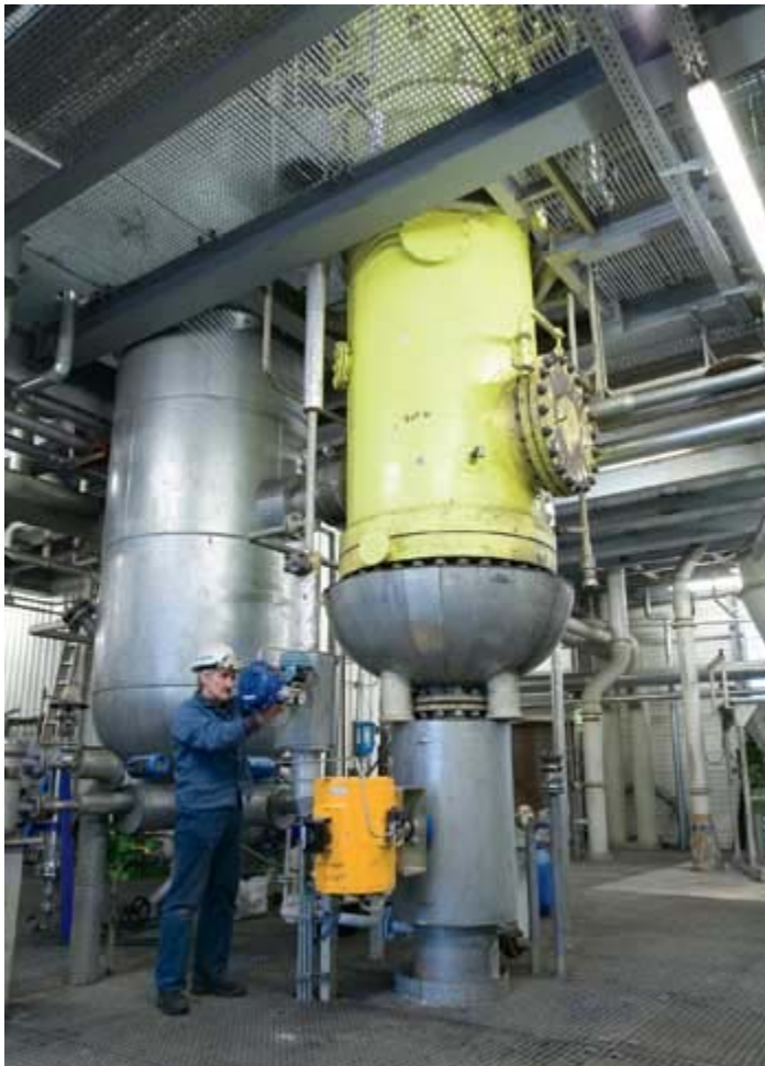
Synthesis gas made from coal is cooled in this chamber by the injection of water. Solidified clinker particles can then be removed and the clean gas sent to a combustor.
